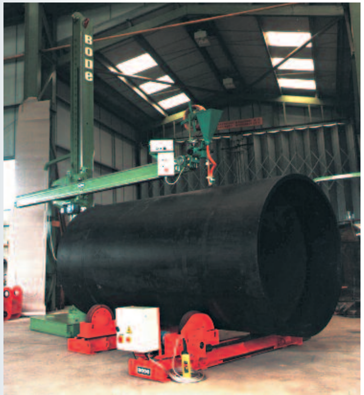
Model 3/TRMB 5 m x 4 m Set-up for seamless pipe welding using submerged arc welding unit.
